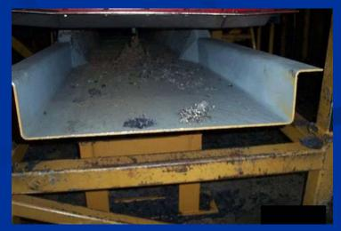
Secondary Granulation 3/4 Inch Being Reduced to 3/8 Inch While Separating Fabric and Steel
