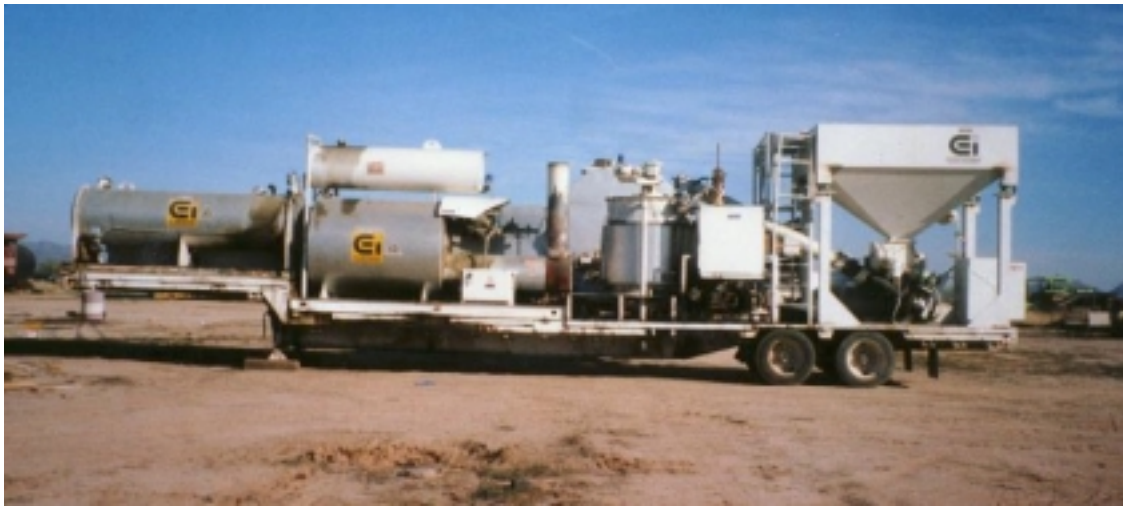
Figure 4 Asphalt rubber blending unit.
