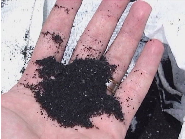
Figure 6. Crumb Rubber after grinding to a 10 mesh or finer.
